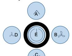
Menu navigation on the touch-surface is performed by pressing the buttons "up" (A), "down" (C), "left" (D), "right" (B) or the power button.
