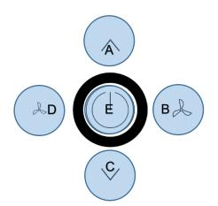
The buttons (A) and (C) change the setpoint in the range ± 3 ° C (default setting, configurable).
